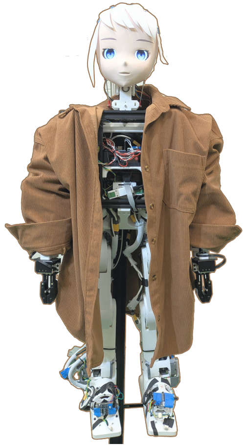
Fig. 16. An anime-style head is integrated into the robot, enabling it to embody expressive and visually appealing anime characters while enhancing its overall aesthetic and potential for engaging human-robot interaction.
